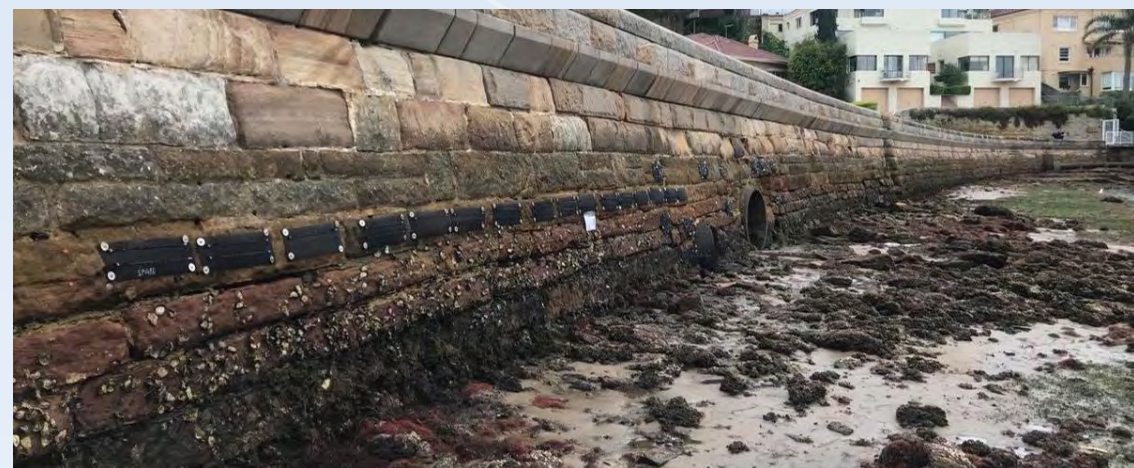
Figure 4. Fibres deployed in marine habitats in Sydney Harbour to investigate rates of chemical, physical and mechanical degradation (work by Bella Charlesworth and Charlotte Beloe, University of New South Wales).
